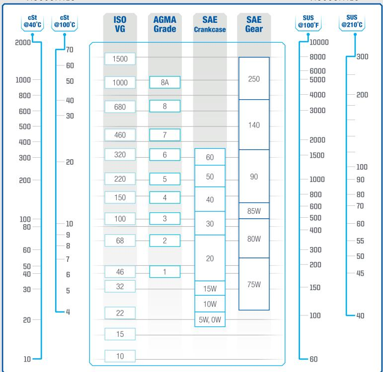
Many petroleum products are graded according to the ISO Viscosity Classification System, approved by the International Standards Organization (ISO). Each ISO viscosity grade number corresponds to the mid-point of a viscosity range expressed in centistokes (cSt) at  $40^{\circ}$ C. For example, a lubricant with an ISO grade of 32 has a viscosity within the range of 28.8 - 35.2, the midpoint of which is 32.
