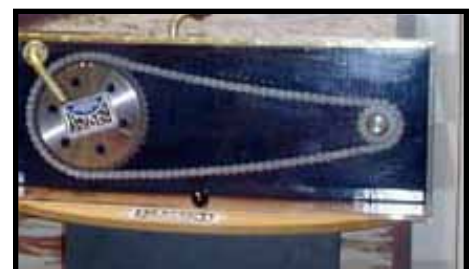
Bel-Ray's German distributor, Meneks, developed this machine that simulates a spinning chain drive. The chain is warmed up, coated with Bel-Ray Super Clean Chain Lube, and allowed to dry. It is then run at speeds in excess of 300kph (186+mph.) The gears are enclosed in a clear, plexiglass case that will show any "fling off"—but to the amazement of the viewer, nothing flings off. This proves the effectiveness of Bel-Ray Super Clean Chain Lube at remaining on the chain, where it belongs.
